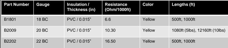
DUPLEX: duplex construction cable made of two solid conductors insulated with various compounds offering a contrasting polarity stripe — eliminate crossover and circuit testing. REDLINE® is a name known to many in the field. This wire is specifically designed for low-voltage connection for any blasting system:
